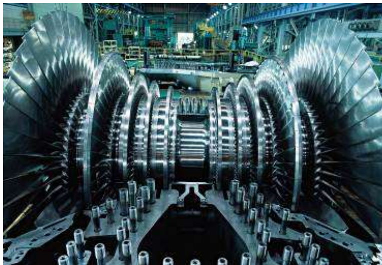
Thermal power turbine
