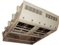
Conversion equipment for the Shinkansen Nozomi N700 series
